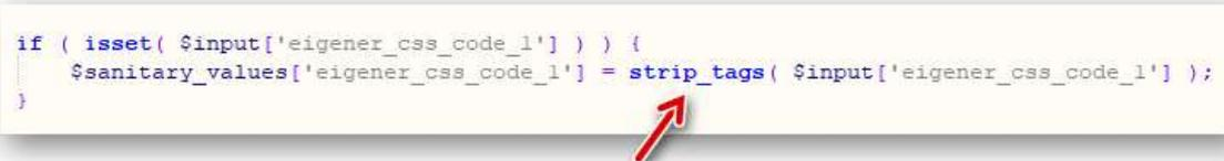
The screenshot shows PHP code for filtering HTML tags in a CSS input field. A red arrow points to the `strip_tags` function call.
